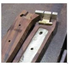
The solution is shown here. Use a small drill press vise (2.5") to hold the pommel perpendicular to the vise's jaws. The whole assembly is then place in a machinist vise and the pommel is pressed to the mating surface. Once the epoxy sets up inside the pommel recesses, there is no way anything can come loose without destroying the handle first.
