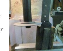
The blade was positioned at a slight angle (because I think it just looks cooler!) and the saw was moved to the left and positioned with the axis of rotation of the saw perpendicular to the tang's dorsal surface (ok – the spine...whatever). The mill was SLOWLY cranked to the left and to create an approximately 3/16° slot.
